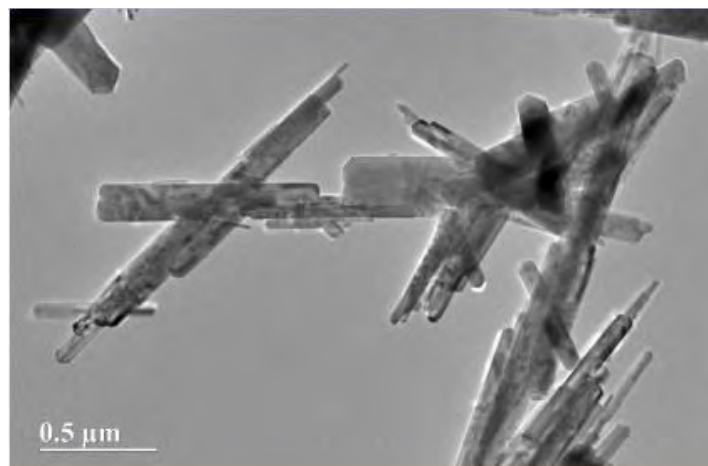
Figure 2 – Microscopic image obtained by transmission electron microscopy (TEM) of a sample of iron oxide used as a yellow pigment in the composition of microconcretes. The irregular and elongated shape of the magnified pigment particles can be seen.
